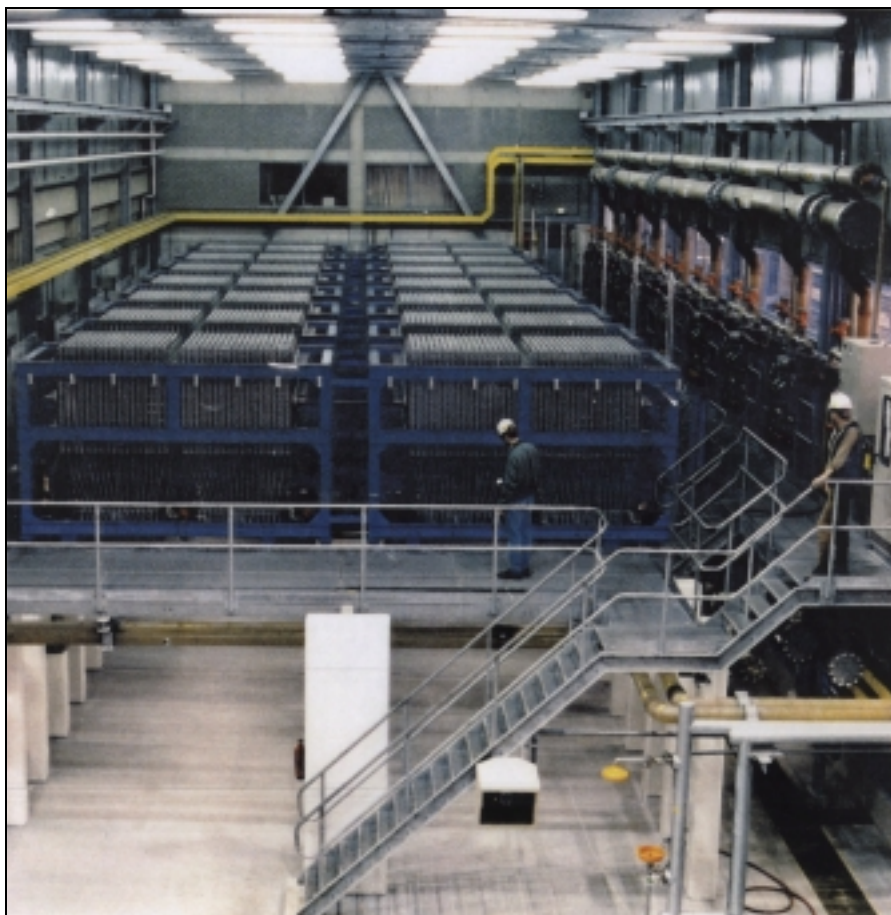
Figure 2.10: View of a membrane cell room equipped with bipolar electrolysers (Source: Hoechst-Uhde)
